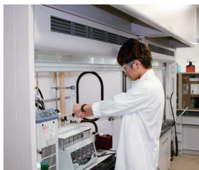
Personal organic synthesizer "ChemiStation" for individual stirring and control of liquid temperature
