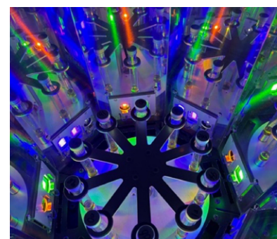
Photochemical apparatus designed for visible-light irradiation in studies of artificial photosynthesis
