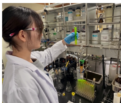
Inspection of a purified fluorescent chemical compound obtained through column chromatographic purification
