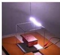
Simulated lightning strike test on lightning protection cage
