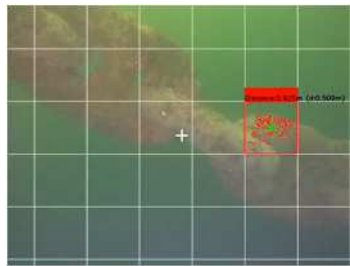
Semi-automatic tracking mooring chain
