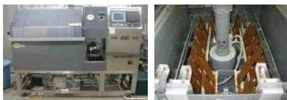
Combined cyclic corrosion test
